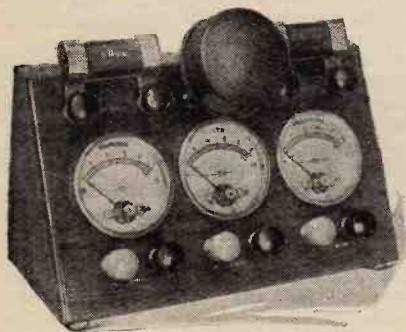
Precision Universal D.C. test set with shunts and series resistance for the voltmeter, in position.
