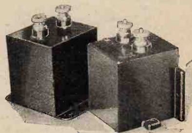
Remoulded T.C.C. 4 mfd condensers. Note the generous size of the terminals.
